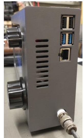
Right side: BNC output connector and USB and Ethernet ports of the Raspberry Pi
